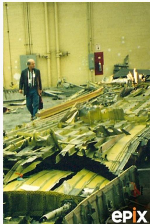
After TWA Flight 800 exploded off Fire Island, investigators collected its damaged parts from the ocean floor and reassembled the Boeing 747 in a hangar at Calverton Airport in Riverhead.
